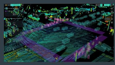
Cities can easily define virtual detection zones for vulnerable road users (VRUs), allowing monitoring of crosswalks, mid-block crossings, and pedestrian behavior. Key detection capabilities include:
